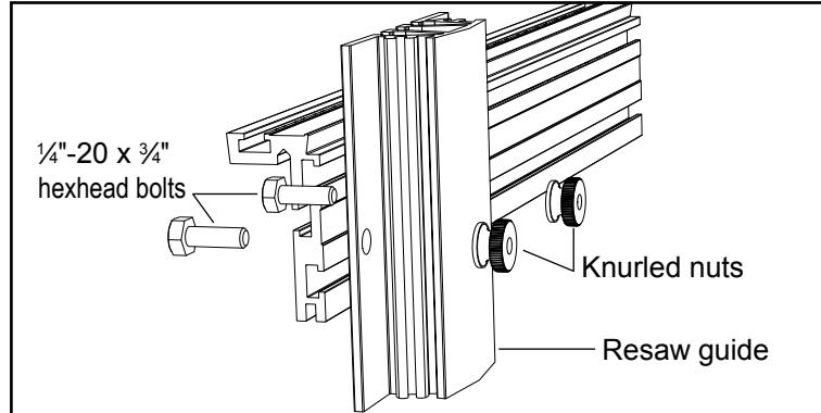
Slide the resaw guide along the fence and position the center of the curved surface  $\frac{1}{4}$ " [6mm] in front of the blade. Tighten the knurled nuts.
